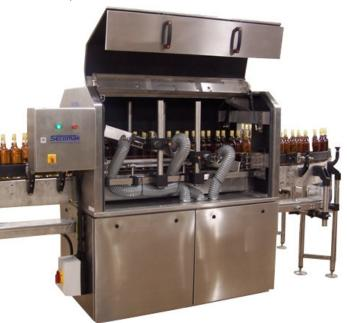
Manufactured from high grade stainless steel the top enclosure, with space saving gull wing doors, contains and directs the dispersed water to ground level via an integral drip tray and drain which also serves to isolate and protect the high efficiency blower.
