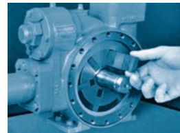
Simple vane replacement requires no special tools.
